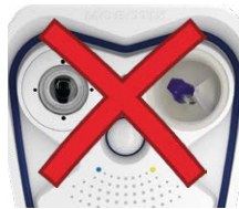
M16 with one transport plug: No operation allowed!
